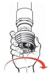
Hand tightening canister may not adequately seat Sprinkler Head, so...
