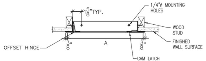
The WBNT No Trim Access Door features a seamless look. An attractive beveled edge door and micro-rounded corners make this an architect favorite. The door features an off-set hinge that allows it to open 180 degrees, while completely hiding the frame from view.
