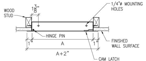
The WB-Basic Access Door is a cost-effective solution, perfect for bidding on any project. This door is manufactured from satincoat galvanized steel, powder coat white and available in a range of popular sizes, ready for installation. It is easily installed using prelocated mounting holes.
