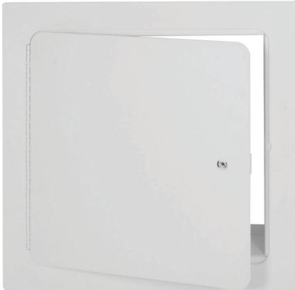
The WB-FR Basic Uninsulated Fire Rated Access Door is designed for wall application only. It is not insulated and should only be installed in environments where temperature rise is not a concern. It features a 1 1/2" trim for an easy flush application into various wall finishes. UL Listed "B" label for 1-1/2 hours. File # R10364C UL US.
