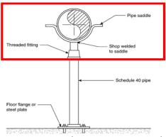
NFPA 13, Section 17.5 Compliant header pipe stands. These stands meet the requirements of NFPA 13, they must however be installed as per section 17.5 to be fully compliant.
