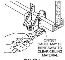
FIGURE 4 MODIFICATIONS REQUIRED TO INSTALL HANGER HEAD SET ON COMPOSITE WOOD JOIST
